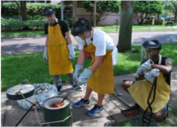
*Center: Paul Perry adds another can to the furnace to be melted down and separated into pure aluminum ingots and waste material called slag. The team goes through hundreds of cans to create several pieces of pure aluminum ingots.*
